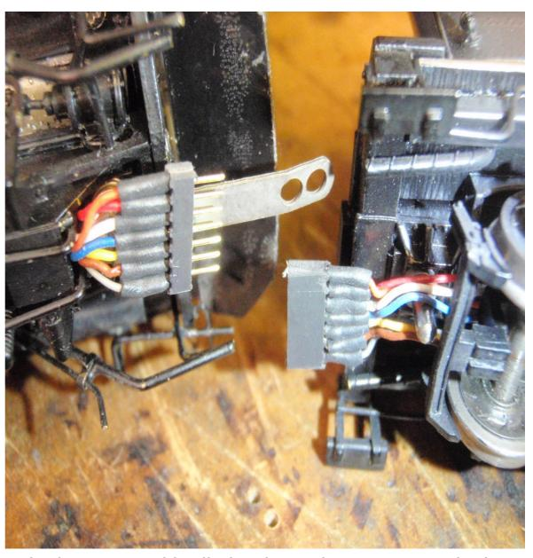
You can also spin the motor with clip leads on the outer two pins!
