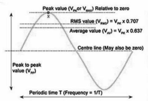
That 1 Vrms sinewave has a peak voltage of 1.414 V, and a peak-to-peak voltage of 2.828 V
