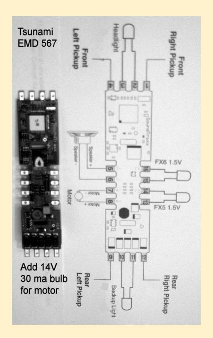
The 14 Volt 30 ma. bulb indicates when there is any motor voltage, without making any sound. Add your 8 ohm speaker, and a small cable for your True RMS meter.
