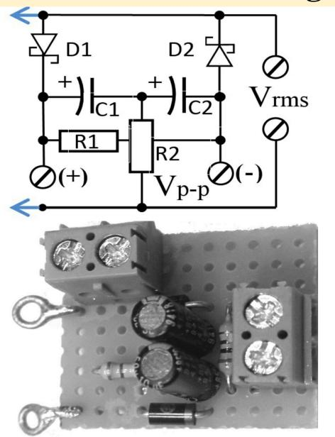
Part No. <a href="http://www.digikey.com/">http://www.digikey.com/</a> MBR160GOS-ND D1, D2 DIODE SCHOTTKY 60V 1A AXIAL P10316-ND C1, C2 CAP ALUM 10UF 50V 20% RADIAL CF14JT1M00CT-ND RES 1M OHM 1/4W 5% CARBON FILM CF14JT220RCT-ND R2 RES 220 OHM 1/4W 5% CARBON FILM 277-1667-ND Vp-p and Vrms TERM BLOCK PCB 2POS 5.0MM 340K-ND BREADBOARD 1/16"DIA 2.00X4.50"
